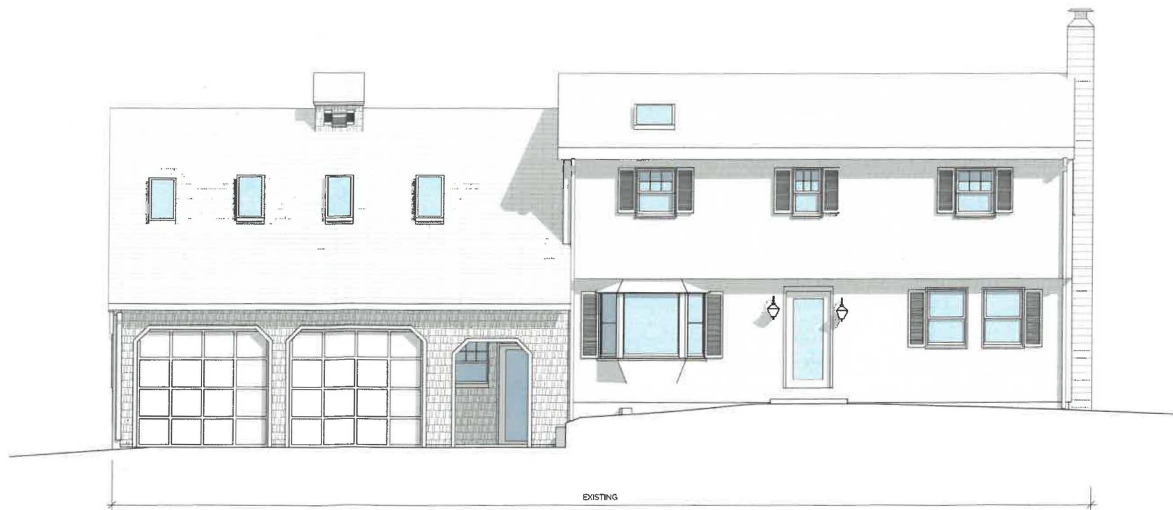
2 EXISTING EAST ELEVATION 1/4" = 1'-0"
